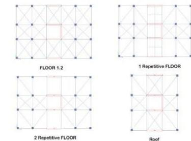
A combination of a braced frame system and a shear-walled frame system consisting of frames, shear walls, diagonal braces are chosen X & V braces, and a outrigger system all of which are put together to effectively resist the seismic force that any direction
